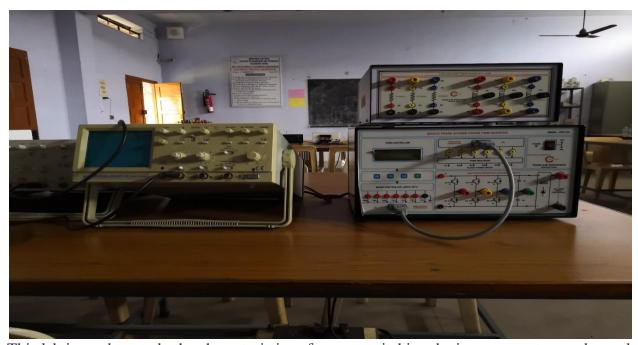
This lab is used to study the characteristics of power switching devices, converters and speed control of electrical machines. This lab also provides the facility to study characteristics of different electronic circuits.
